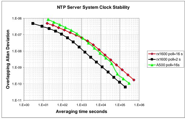
Note the improved stability resulting from decreasing the NTP refclock poll interval from the nominal 16 seconds to 2 seconds, where the standard deviation of the NTP loopstats (system clock offset from PCI bus clock) decreased from  $54 \mu s$  to  $7 \mu s$ . A loopstats histogram is shown below.
