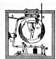
HOW THE BALL IS DROPPED A rope, R, rnns up through a flagstaff, out at top, down to ball at base; windlass, W, lifts the ball to top of pole; Observatory clock sends a current through magnet, M, by which armature, A, is instantly lowered; lever, L, held back by resting against end of armature, is now freed; spring, S, jerks it forward, knocks pawl, P, out of ratchet and ball comes down.
