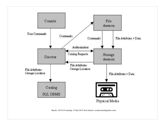
How the components interact. The lines are TCP/IP connections, except the Storage Daemon to Physical Media.
